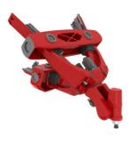
Exechon has solved this problem by connecting the outer gimbles of actuator one and three, eliminating the need of central support of these gimbles and at the same time making it possible to add on extra material in the centre, which was impossible in the platform design due to cable issues, resulting in increased stiffness.
