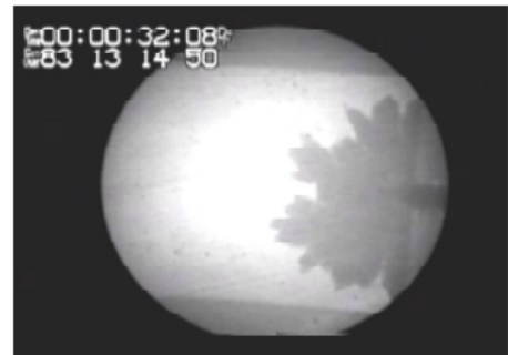
Figure 7: X-ray image for filling 8-mm thick pattern. The rapid, irregular metal flow is evidence of collapse mode.
